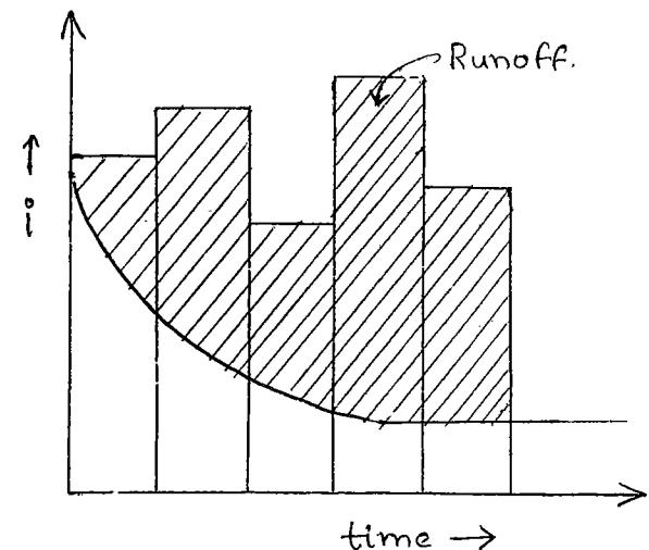
$$\begin{aligned} \text{Total rainfall} &= i_1(t_1 - 0) + \\ &i_2(t_2 - t_1) + i_3(t_3 - t_2) \\ &+ i_4(t_4 - t_3) + i_5(t_5 - t_4). \end{aligned}$$
