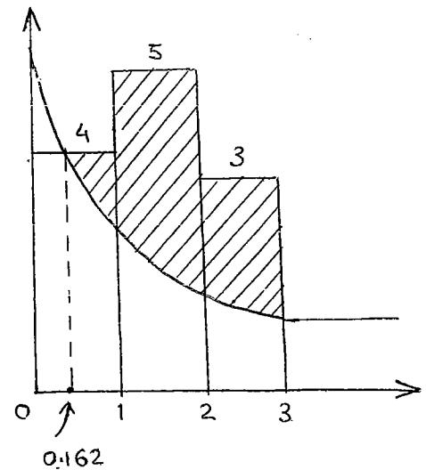
$$\begin{aligned} &= \sum_{t=0.162}^3 i_i t_i - \int_{0.162}^3 f_{ct} dt \\ &= (4 \times 0.838 + 5 \times 1 + 3 \times 1) - \int_{0.162}^3 (1.2 + 4 \cdot 2 e^{-2.5t}) dt \\ &= \underline{\underline{6.8627 \text{ cm}}} \end{aligned}$$
