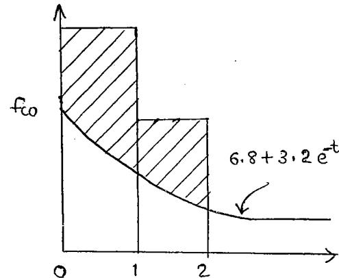
$$\begin{aligned} \text{Runoff} &= \text{rainfall} - \text{infiltration} \\ &= 20 \times 1 + 10 \times 1 - \int_0^2 (6.8 + 3.2 e^{-t}) dt \\ &= \underline{\underline{13.63}} \end{aligned}$$
