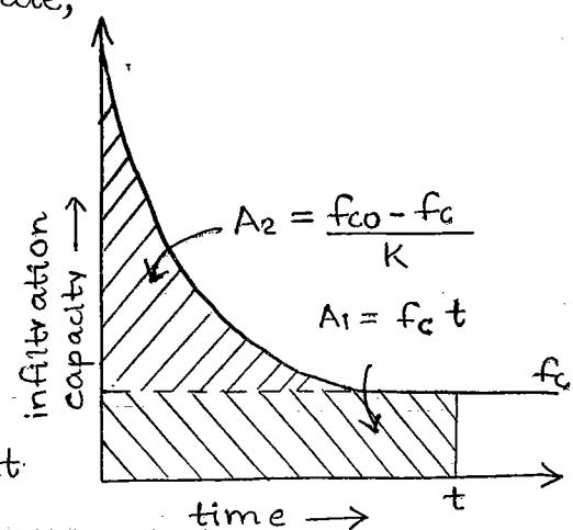
○ At any time  $t$ ,  $f_{ct} > f_c$ , soil yet to attain steady state
