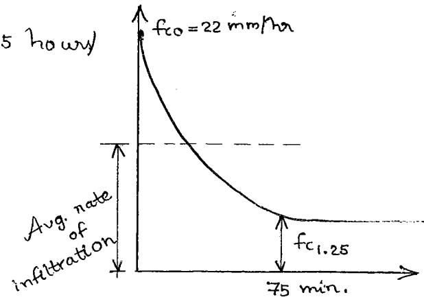
$\therefore$  Average infiltration rate for first 75 min = total infiltration / time
