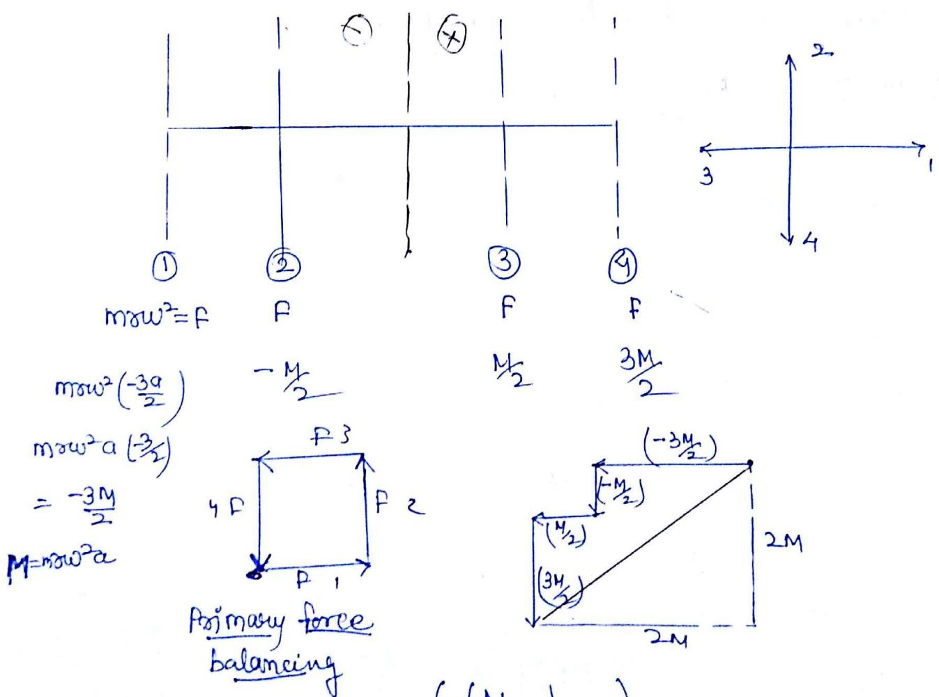
$$\left( \left( M_{\text{net}} \right)_{\text{primary}} \right)_{\text{max}} = 2\sqrt{2} M$$
