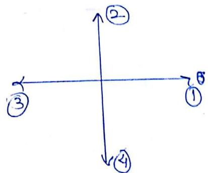
$$(F_{net})_{\text{primary}} = m \omega^2 [ \cos \theta + \cos(90^\circ + \theta) + \cos(180^\circ + \theta) + \cos(270^\circ + \theta) ]$$
