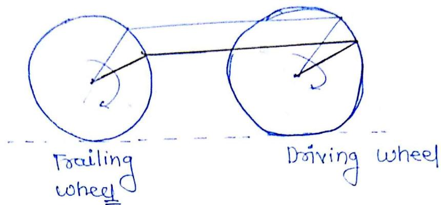
Coupling rod was basically introduced to decrease the amount of hammer blow by decrease the balance mass requirement in order to balance the reciprocating mass of the cylinder through splitting the reciprocating b/w the driving wheel & trailing wheel this was the development from the passenger locomotive to express locomotive in which two - two wheels are coupled to the super fast locomotive in which three - three wheel were coupled.
