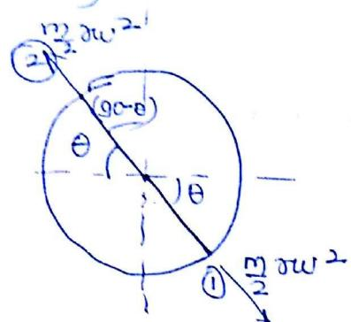
$$(F_{\text{net}})_{\text{primary}} = m\omega^2$$
