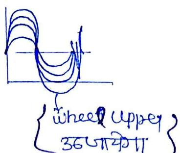
$$\text{load on wheel} = \text{static load} + B b w^2 \sin \theta$$
