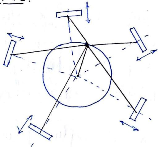
In Radial engines there is only single crank and whose plane of rotation remains same for all the cylinder so there is no unbalanced primary & secondary moment or couple.
