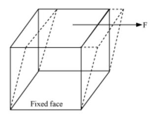
• Strain : Deformation amount/original dimension  $\left(\frac{\Delta L}{L}, \frac{\Delta V}{V}\right)$
