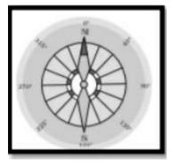
(vi) Direction of a place can be found out with the help of an instruement called Compass.Its magnetic needle always points towards the North-South direction.
