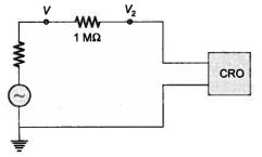
If  $V_1 = 5$  V and  $V_2 = 3$  V, then what is the input impedance of the CRO in the above circuit?
