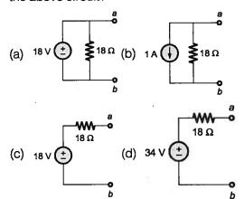
In the following circuit the value of open circuit voltage and Thevenin resistance at terminals a, b are
