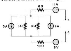
Which of the following circuit is equivalent to the above circuit?
