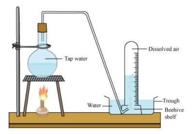
Heat the water in the round bottomed flask. After some time, some tiny bubbles of gas coming out of the water are observed. If the heating is continued, then water starts boiling and the gas bubbles start coming out of the beehive shelf.
