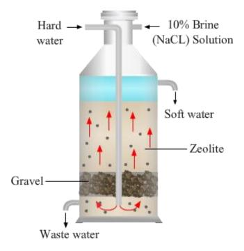
(iii) In the column given in the figure, sand, gravel and permutit are placed in alternate layers through which hard water flows down. As water passes, Ca<sup>2+</sup> and Mg<sup>2+</sup> ions are exchanged with Na<sup>+</sup> ions of the permutit. This forms calcium and magnesium permutit leaving behind only pure water.
