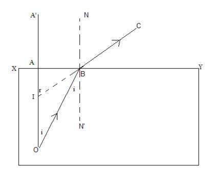
In figure, OA passes straight along OAA'. Another ray of light from O incident at angle i on XY along OB deviates away from normal. It gets refracted at angle r along BC. When we produce back BC meets OA at I. Hence it's the virtual image of O. Hence AI is the apparent depth and AO is the real depth.
