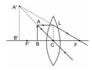
The image formation of an object AB placed between the optical centre C and principal focus F' of a convex lens has been shown in fig. The image A'B' is virtual, erect and magnified.
