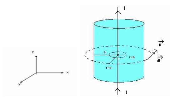
As the magnetic field lines form closed circle, so the magnetic field is tangential to the loop everywhere, and is in the same direction as dl taken in the counter clock wise direction. Thus, the angle between the magnetic field and dl is zero everywhere on the loop.
