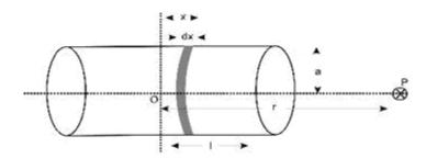
The magnitude of the field at point P due to the circular element is,
