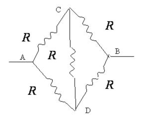
It is a balanced Wheatstone bridge. Therefore, point C and D are at the same potential. Since no current flows in the branch CD, this branch is ineffective in determining the equivalent resistance between terminal A and B and can be removed.
