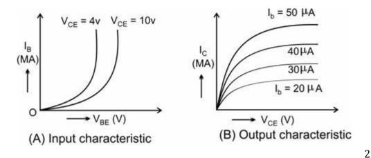
Output Characteristics: Keep value of base current  $I_b$  fixed with the help of  $V_{BE}$ . Now gradually change the value of  $V_{CE}$  and note the values of collector current  $I_C$ . Plot  $I_C - V_{CE}$  graph. Repeat the process for different constant values of  $I_b$ . The output characteristics are shown in fig\_(b).
