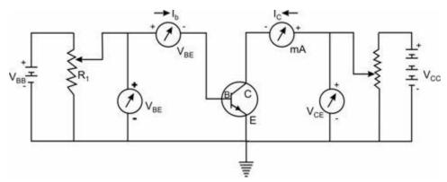
Input Characteristics: Adjust collector-emitter voltage  $V_{CE}$  with the help of rheostat  $R_2$  and set it at a fixed value  $V_{CE}$ . Now with the help of rheostat  $R_1$  gradually increase the value of base-emitter voltage  $V_{BE}$  in small steps and note the corresponding values of base current  $I_b$ .
