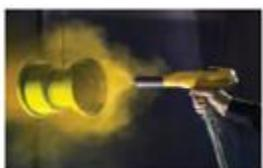
**Answer :** The picture depicts of the powder coating i.e. powder is sprayed on the polished metal surface by electrostatic spray deposition.
