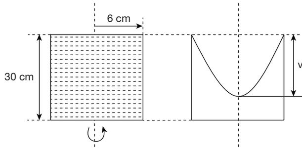
$$y = \frac{\omega^2 r^2}{2g} \Rightarrow y = \left[ \frac{2\pi \times 300}{60} \right]^2 \times 0.06^2 \times \frac{1}{2 \times 9.81}$$
