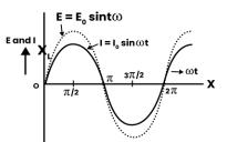
a.c. circuit having R only, as current and voltage are in the same phase, hence in fig. both phasors  $E_0$  and  $I_0$  are in the same direction, making an angle  $\omega t$  with OX. Their projection on Y-axis represent
