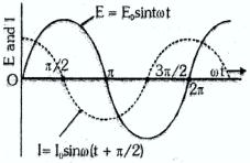
The two plates of the capacitor become alternately positively and negatively charged and the magnitude of the charge on the plates of the capacitor varies sinusoidally with time. Also the electric field between the plates of the capacitor varies sinusoidally with time. Let at any instant t charge on the capacitor =  $\mathbf{q}$
