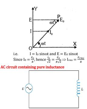
A circuit containing a pure inductance L (having zero ohmic resistance) connected with a source of alternating emf. Let the alternating e.m.f.  $E = E_0 \sin \omega t$
