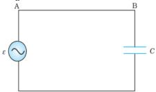
When alternating e.m.f. is applied across the capacitor a similarly varying alternating current flows in the circuit.
