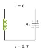
The moment the circuit is completed, the charge on the capacitor starts decreasing, giving rise to current in the circuit. Let q and i be the charge and current in the circuit at time t. Since di/dt is positive, the induced emf in L will have polarity as shown, i.e.,
