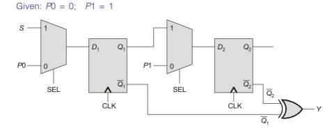
Output,  $Y = \overline{Q_2} \oplus \overline{Q_1}$  ...(i)
