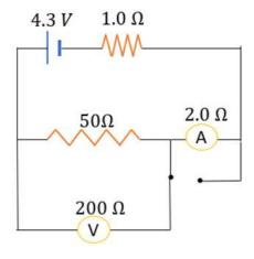
We will treat the measuring devices as ordinary resistors. Now, voltmeter and  $R=50\Omega$  are in parallel. The equivalent resistance is given by:
