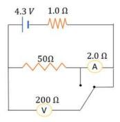
We will treat the ammeter and the voltmeter as ordinary resistors to find the equivalent resistance.
