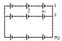
When  $n_1$  cells each with emf 'E' are connected in series, the total emf,  $E_{\text{net}}$  in one branch is,
