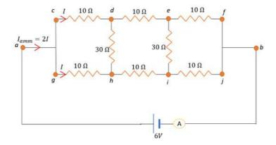
Due to this symmetry, d and h; e and i are the same potential. Hence, no current passes through *de* and *ei*.
