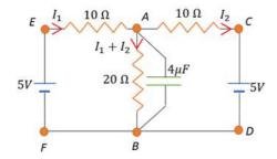
At steady state, no current passes through the capacitor; hence, the results are the same as in (a).
