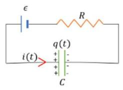
Let the potential across the capacitor be at time t be  $V_c$ . Let the charge at time t be q. The initial charge is Q.
