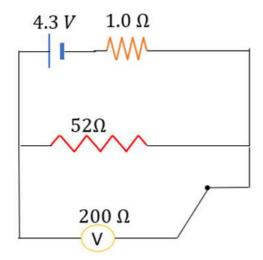
Note that the voltmeter and r' are in parallel.
