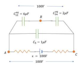
Now, the two capacitors  $C_{12}^{eq}$  and  $C_{34}^{eq}$  are in series.
