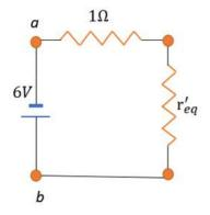
Now, the 1  $\Omega$  resistor and  ${r^{\prime}}_{eq}$  are in series.
