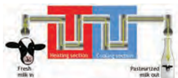
Fig 4.9: Pasteurisation of milk
