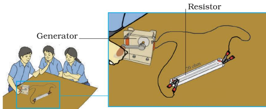
**Fig. 7.11.1** Generator connected to a resistor
