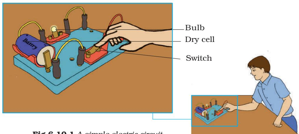
**Fig.6.10.1** A simple electric circuit
