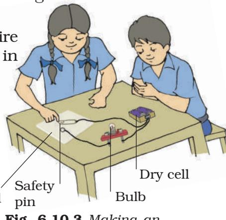
**Fig. 6.10.3** Making an electric switch
