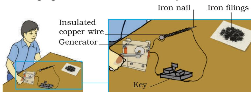
**Fig.7.11.3** An electromagnet
