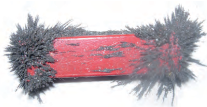
Fig. 13.7 Iron filings sticking to a bar magnet
