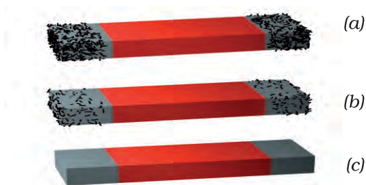
Fig. 13.6 Magnet with (a) many iron filings (b) few iron filings and (c) no iron filings sticking to it.
