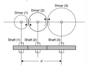
$d = R_1 + 2R_2 + R_3$ , with one idler. This formula holds good only when all the three shafts are parallel and centres of gears are on same straight line.
