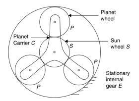
An epicyclic gear train consists of a sun wheel *S*, a stationary internal gear *E* and three identical planet wheels *P* carried on a star shaped carrier *C*. The size of the different toothed wheels are such that the planet carrier *C* rotates at  $\frac{1}{4}$  of the speed of the sun wheel *S*. The minimum number of teeth on any wheel is 18. The driving toque on the sun wheel is 80 N m.
