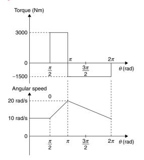
The torque and the angular speed data over one cycle for a shaft carrying a flywheel are as shown in the above figures. The moment of inertia (in kg  $m^2$ ) of the flywheel is
