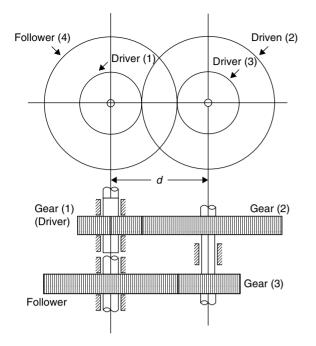
In the reverted gear train shown, the driver (gear 1) and the follower (gear 4) are co-axial. The intermediate shaft mounts gears 2 and 3 on it.
