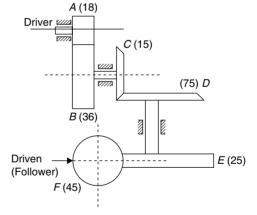
A compound gear train consists of spur, bevel and spiral gears as is shown in the figure with the name of gear in bold capital letters followed by the number of teeth on that gear in parenthesis (bracket). Gear A is the driver and gear F is the driven (follower). The overall speed ratio of the train is
