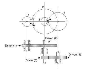
A compound gear train is shown in figure. Gears 2 and 3 are mounted on the same shaft (intermediate shaft). Hence, gear 2 and gear 3 rotate with the same angular velocity, in the same sense of rotation.
