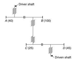
In the compound gear train shown, gears B and C are mounted on the same shaft, gear A is mounted on the driving shaft which rotates at 1170 rpm in the clockwise sense. The table below gives the number of teeth on each gear.
