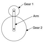
If the arm is fixed, then gear 1 and gear 2 can only rotate about their fixed axes and in such a case it becomes a simple gear train. But if either gear 1 is fixed (or only gear 2 is fixed), then the arm connecting the gears can also move and the arrangement becomes an epicyclic gear train. The fixed gear becomes 'the Sun' and the moving gear becomes the planet. The whole arrangement can be enclosed is an annual wheel, which can be fixed (instead of fixing the gears).
