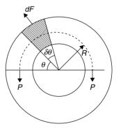
Consider a small element of rim as shown in figure. Volume of the element =  $A \times R \ \delta\theta$ where A = area of cross section Mass of the element  $dm = \rho \ A \ R \ \delta\theta$ where  $\rho$  = density, R = means radius of rim Centrifugal force  $dF = dm \ \omega^2 R$  $= \rho \ A \ R^2 \ \delta\theta \ \omega^2$
