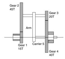
A planetary gear train has four gears and one arm (carrier). Angular velocities of the gears are  $\omega_1$ ,  $\omega_2$ ,  $\omega_3$  and  $\omega_4$  respectively. The carrier rotates with angular velocity  $\omega_5$ .
