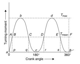
As work done is the product of the turning moment and the angle turned, the area of the turning moment diagram represents the work done per revolution.
