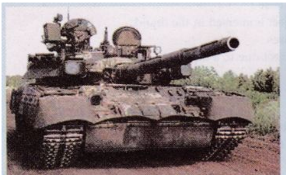
A wide steel belt is provided over the wheels of an army tank.
