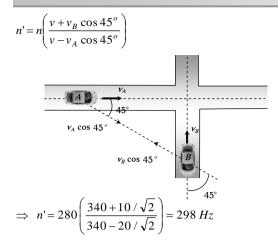
14. (b) For observer note of B will not change due to zero relative motion.
