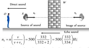
The other sound is echo, reaching the observer from the wall and can be regarded as coming from the image of source formed by reflection at the wall. This image is approaching the observer in the direction of sound.
