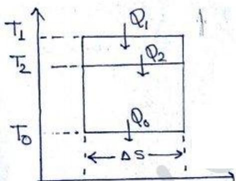
$$\eta = \frac{\text{output}}{\text{Input}} = \frac{W_{\text{net}}}{Q_S} = \frac{Q_{\text{net}}}{Q_S} = \frac{Q_S - Q_R}{Q_S}$$
