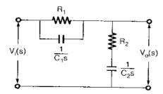
$$\frac{V_o(s)}{V_i(s)} = \frac{\alpha(1 + T_1 s) (1 + T_2 s)}{(1 + \alpha T_1 s) (1 + \beta T_2 s)}$$
