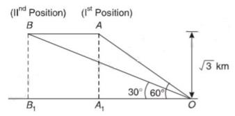
For  $\Delta OB_1$ , B,  $OB_1 = \sqrt{3} \tan 30^\circ = 3 \, \mathrm{km}$ As, a distance of  $3-1=2 \, \mathrm{km}$  is covered in 5 seconds. Therefore the speed of the plane is  $\frac{2 \times 3600}{5} = 1440 \, \mathrm{km}$  / hr
