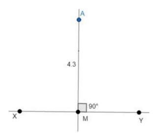
Step3: now using protractor draw lines at angles at 30° to the left of A and 30° to the right of A and mark the intersection points with line XY as B and C respectively thus required  $\Delta ABC$  is ready
