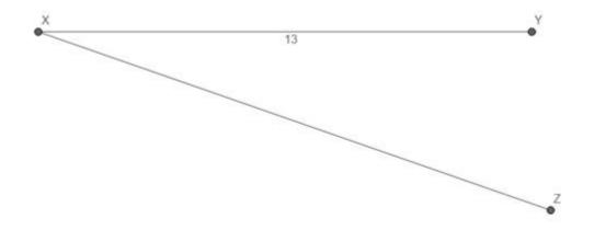
Step3: take any distance in compass and keeping the needle of the compass on point X cut an arc on line XZ and name that point  $X_1$ . Keeping the distance in compass same keep the needle of the compass on point  $X_1$  and cut an arc on line XZ and mark that point as  $X_2$ . By doing this we are diving the line XZ in equal parts. Divide line into 2+3+4 = 9 parts i.e. by repeating this process mark points to  $X_9$
