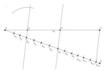
Step7: take distance RY in compass keep the needle at point R and draw an arc intersecting the arc drawn in step6 mark the intersection point as point P. draw segments PQ and PR and required  $\Delta$ PQR is ready
