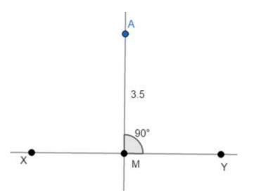
Step3: now using protractor draw lines at angles at 30° to the left of A and 30° to the right of A and mark the intersection points with line XY as B and C respectively thus required  $\Delta$ ABC is ready
