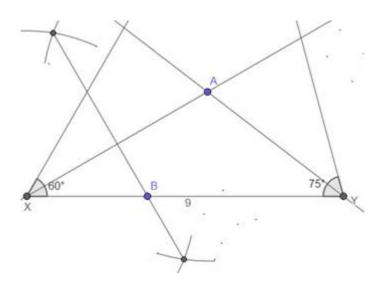
Step5: similarly draw perpendicular bisector of segment AY and mark the intersection point with XY as C join AB and AC and required  $\Delta$ ABC is ready
