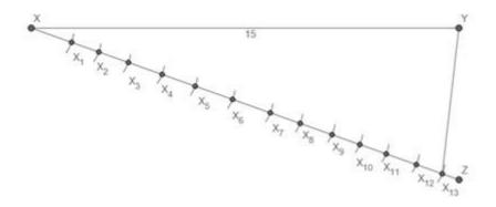
Step5: as the ratio is 3:4:6 consider 3 parts i.e. point  $X_3$  then 4 parts i.e. point  $X_7$  and then 6 parts i.e. point  $X_{13}$  construct lines from point  $X_3$  and  $X_7$  parallel to line  $YX_{13}$  intersecting line XY at points Q and R respectively
