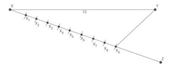
Step5: as the ratio is 2:3:4 consider 2 parts i.e. point  $X_2$  then 3 parts i.e. point  $X_5$  and then 4 parts i.e. point  $X_9$  construct lines from point  $X_2$  and  $X_5$  parallel to line YX<sub>9</sub> intersecting line XY at points Q and R respectively
