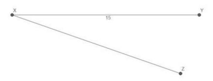
Step3: take any distance in compass and keeping the needle of the compass on point X cut an arc on line XZ and name that point  $X_1$ . Keeping the distance in compass same keep the needle of the compass on point  $X_1$  and cut an arc on line XZ and mark that point as  $X_2$ . By doing this we are diving the line XZ in equal parts. Divide line into 3+4+6 = 13 parts i.e. by repeating this process mark points to  $X_{13}$
