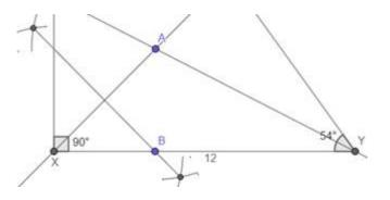
Step5: similarly draw perpendicular bisector of segment AY and mark the intersection point with XY as C join AB and AC and required  $\Delta$ ABC is ready
