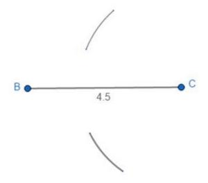
Step3: keeping the distance in the compass same as in the above step keep the needle of compass on point B and draw arcs intersecting the previous arcs above and below BC. Mark the intersection points of arcs as M and N
