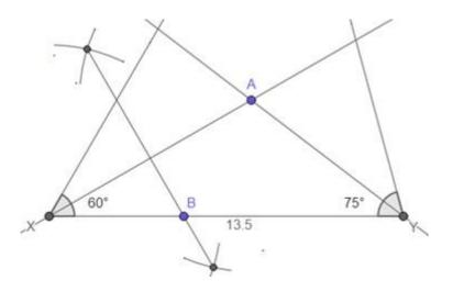
Step5: similarly draw perpendicular bisector of segment AY and mark the intersection point with XY as C join AB and AC and required  $\Delta$ ABC is ready
