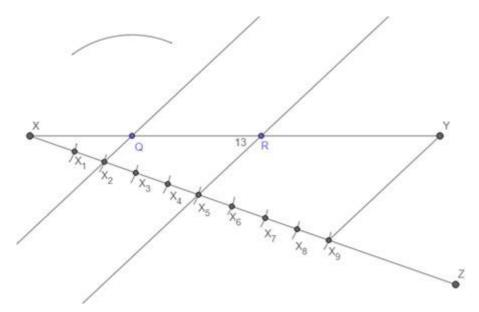
Step7: take distance RY in compass keep the needle at point R and draw an arc intersecting the arc drawn in step6 mark the intersection point as point P. draw segments PQ and PR and required  $\Delta$ PQR is ready
