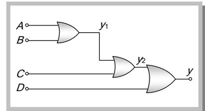
70. What is the output of the combination of the gates shown in the fig.
