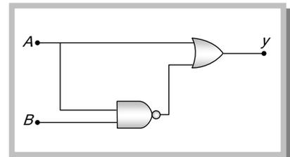
71. In circuit in following fig. the value of  $Y$  is
