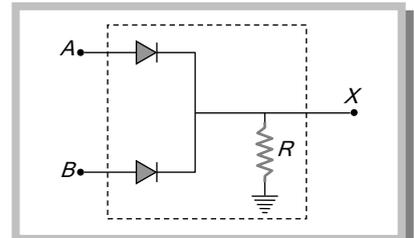
76. The circuit shown in fig. is used to realise a logic gate. The gate is
