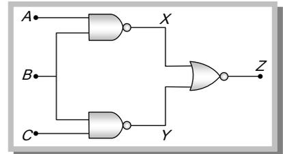
78. The Boolean expression for the output  $f$  of the combination of logic gates shown in fig. is
