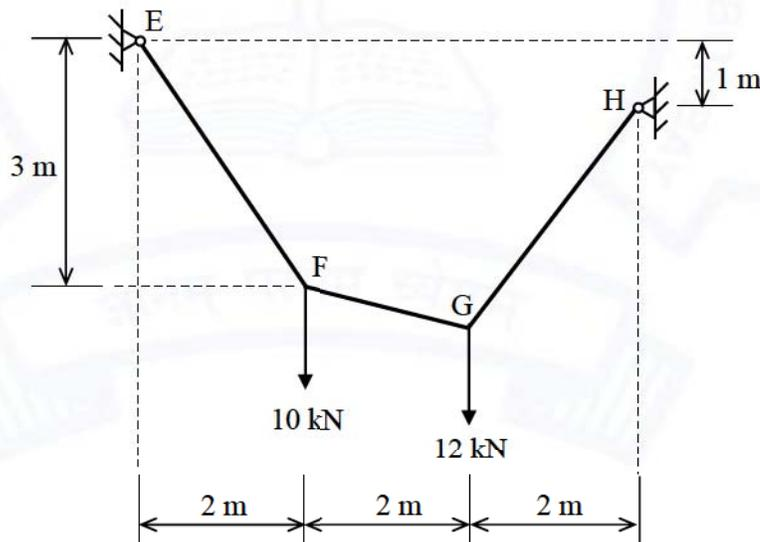
The magnitude of tension in the cable segment FG (in kN, round off to two decimal places) is \_\_\_\_\_
