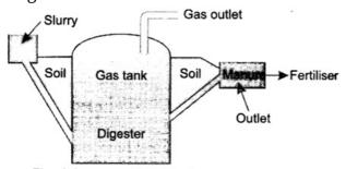
Fixed dome type biogas plant
