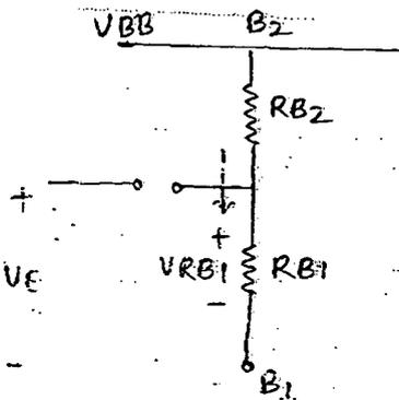
$$V_{RB1} = \left( \frac{R_{B1}}{R_{B1} + R_{B2}} \right) V_{BB}$$
