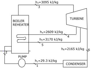
kJ/kg). After expansion in the turbine to 400 kPa ( $h_4 = 2609 \text{ kJ/kg}$ ), the steam is reheated to  $350^{\circ}$ C ( $h_5 = 3170 \text{ kJ/kg}$ ), and then expanded in a low pressure turbine to 10 kPa ( $h_6 = 2165 \text{ kJ/kg}$ ). The specific volume of liquid handled by the pump can be assumed to be
