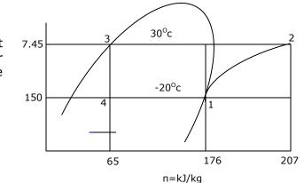
condensing temperature of 30°C and evaporator temperature of -20°C. The clearance volume ratio of the compressor is 0.03. Specific heat ratio of the vapour is 1.15 and the specific volume at the suction is 0.1089 m<sup>3</sup>/kg. Other properties at various states are given in the figure. To realize 2 Tons of refrigeration, the actual volume displacement rate considering the effect of clearance is
