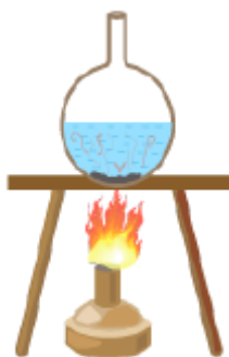
Figure 1: Transfer of heat by convection in water
