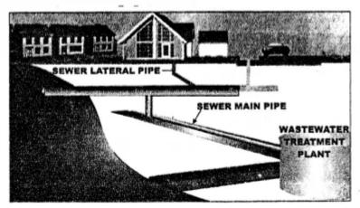
2. **Water treatment plant:** The waste water from sewer main pipe is then led to the water treatment plant.
