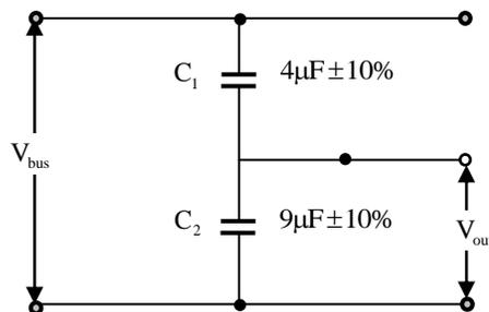
The measurement capacitors  $C_1$  and  $C_2$  have tolerances of  $\pm 10\%$  on their nominal capacitance values. If the bus voltage  $V_{bus}$  is 100 kV rms, the maximum rms output voltage  $V_{bus}$  (in kV), considering the capacitor tolerance, is \_\_\_\_\_.
