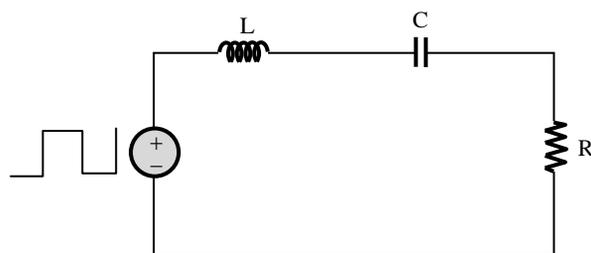
The amplitude of the  $5000\text{ rad/s}$  component of the capacitor voltage (in volt) is \_\_\_\_\_.
