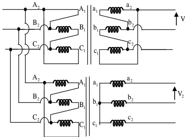
The phase difference (in degree) between voltage  $V_1$  and  $V_2$  is \_\_\_\_\_.
