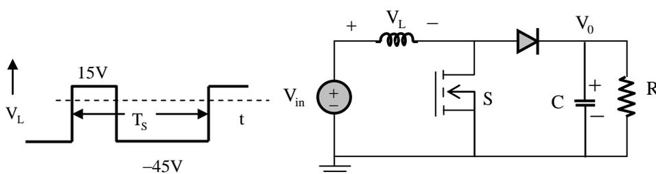
Also assume that the components are ideal, the inductor current is always positive and continuous and switching period is  $T_s$ . If the voltage  $V_L$  is as shown, the duty cycle of the switch  $S$  is \_\_\_\_\_.
