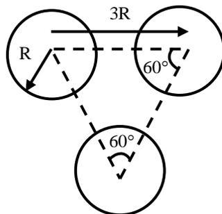
The geometric mean radius (GMR) (in cm) of the composite conductor is  $kR$ . The value of k is \_\_\_\_\_.
