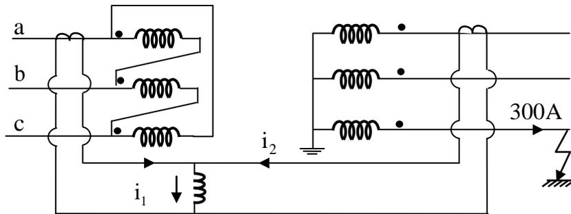
The current transformers (CTs) on low and high voltage sides have a ratio of 500/5. Find the currents  $i_1$  and  $i_2$ , if the fault current is 300A as shown in figure.
