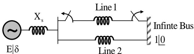
If one line is tripped at time  $t_1$  by opening the circuit breakers at the two ends (although there is no fault), then it is seen that the generator undergoes a stable transient. Which one of the following waveforms of the rotor angle  $\delta$  shows the transient correctly?
