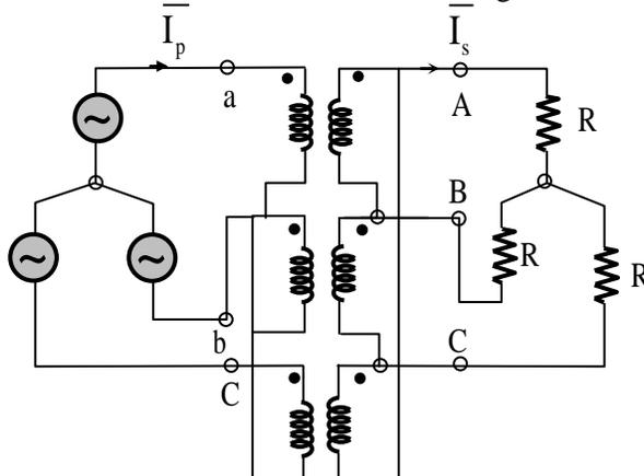
The line-to-line voltage rating is 230 V on the star side, and 115 V on the delta side. If the magnetizing current is neglected and  $\bar{I}_s = 100\angle 0^\circ$  A, then what is the value of  $\bar{I}_p$  in Ampere?
