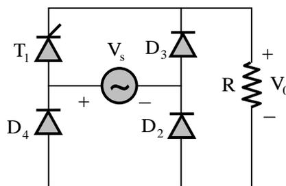
If the input voltage  $V_s$  is  $100 \sin(100\pi t)$  V, the average voltage across R (in Volt) under steady-state is \_\_\_\_\_.
