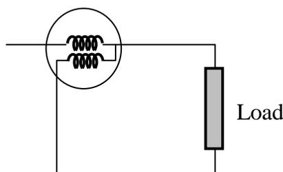
The wattmeter is connected as shown in the figure, to measure the power consumed by a load, which draws 25A at power factor 0.8. The voltage across the load terminals is 30V. The percentage error on the wattmeter reading is \_\_\_\_\_.
