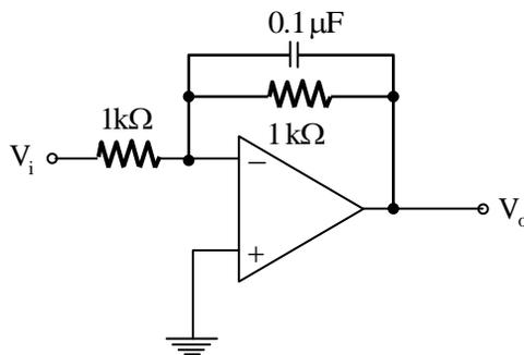
The amplitude of the output voltage  $V_o$  (in Volt) is \_\_\_\_\_.
