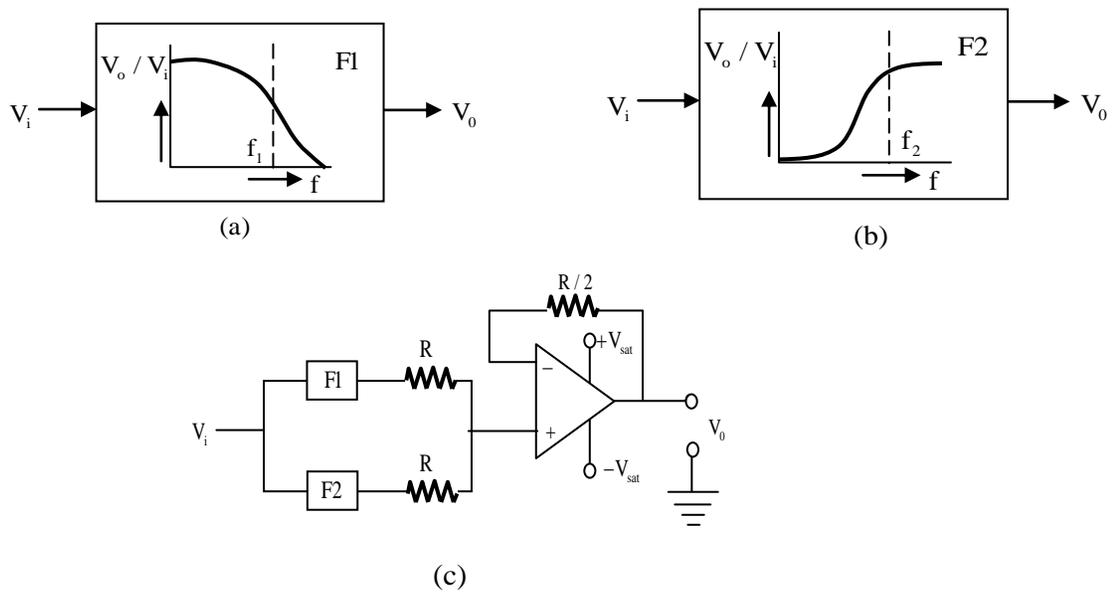
The cut-off frequencies of F1 and F2 are  $f_1$  and  $f_2$  respectively. If  $f_1 < f_2$ , the resultant circuit exhibits the characteristics of a
