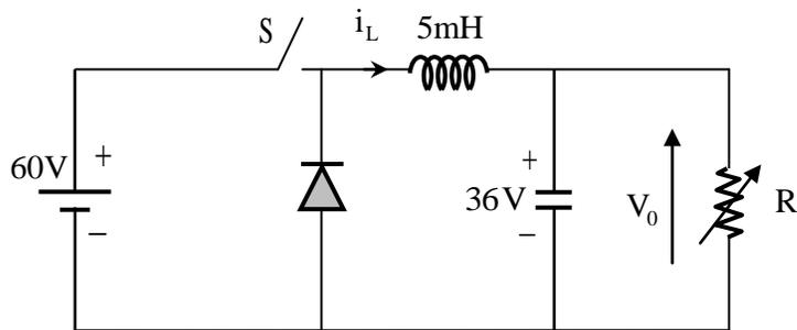
The output voltage  $V_0$  is 36V. Assume that all the components are ideal, and that the output voltage is ripple-free. The value of R (in Ohm) that will make the inductor current ( $i_L$ ) just continuous is \_\_\_\_\_.
