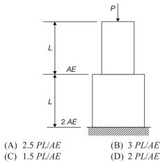
8. The total elongation of the structural element fixed, at one end, free at the other end, and of varying cross-section as shown in the figure when subjected to a force *P* at free end is given by
