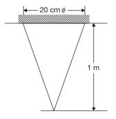
If specific weight is 80000 N/m<sup>3</sup> and modulus of elasticity is,  $E = 2 \times 10^5$  N/mm<sup>2</sup>, then extension of its length due to self weight is
