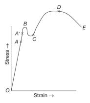
In the initial portion OA, stress is directly proportional to strain. Point A is the limit of proportionality. Slightly beyond A, when the load is released, strain disappears completely and original length is regained.
