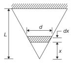
Consider an element of length dx and diameter d at a distance x from the free end.
