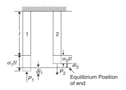
Free expansion of bar  $1 = \alpha_1 t L$ Free expansion of bar  $2 = \alpha_2 t L$
