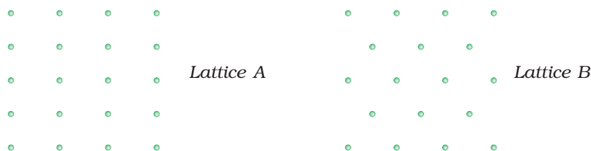
Fig. 1.6: Arrangement of points in two different lattices
