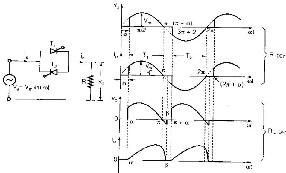
□ RMS value of output voltage for R load
