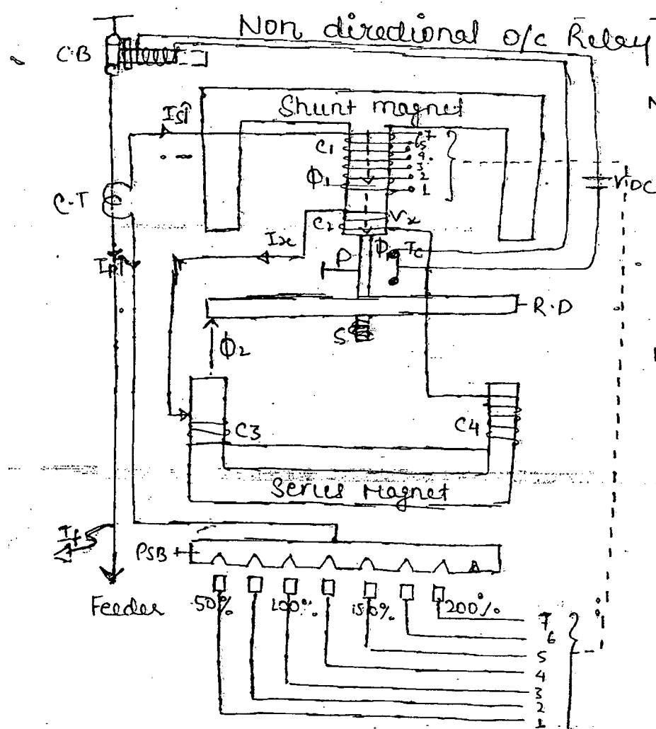
N.B: For measurement of current we use series magnet
