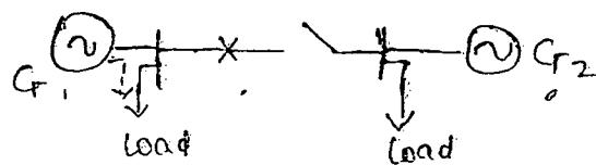
Non-directional over current (O.C) relay is produced trip signal. If the fault current If magnitude is more than relay internal setting value and it is independent from fault current dir. So it is called non directional. It is practically use to source end to identify the fault to the source side & line side.
