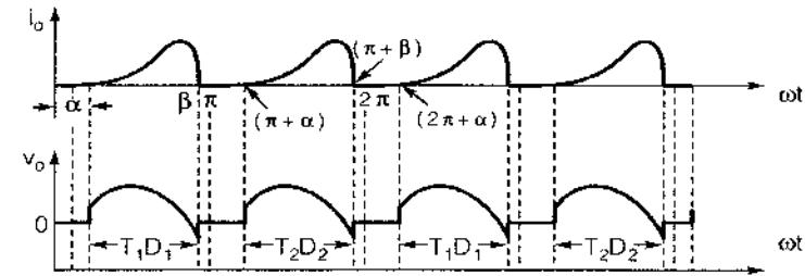
(b)  $\beta < \pi$  and  $V_m \sin \beta < E$  (Discontinuous conduction)
