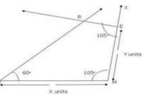
• A quadrilateral can be constructed uniquely if its three sides and two included angles are given.
