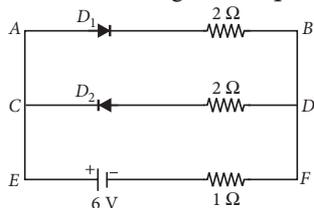
$D_2$  will be reversed biased and  $D_1$  will be forward biased so equivalent circuit will be
