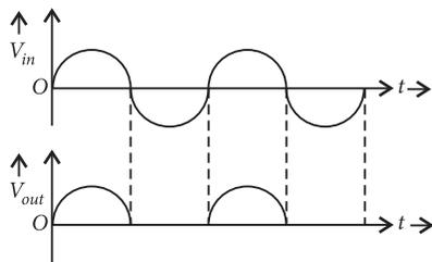
During negative half cycle of input a.c., end  $A$  of the secondary winding becomes negative and end  $B$  positive. Thus, diode  $D$  becomes reverse biased and does not conduct any current. So, no current flows in the circuit. Since electric current through load  $R_L$  flows only during positive half cycle, in one direction only *i.e.*, from  $A$  to  $B$ , so d.c. is obtained across  $R_L$ .
