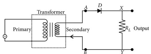
It consists of a diode  $D$  connected in series with load resistor  $R_L$  across the secondary windings of a step-down transformer. Primary of transformer is connected to a.c. supply. During positive half cycle of input a.c., end  $A$  of the secondary winding becomes positive and end  $B$  negative. Thus, diode  $D$  becomes forward biased and conducts the current through it. So, current in the circuit flows from  $A$  to  $B$  through load resistor  $R_L$ .
