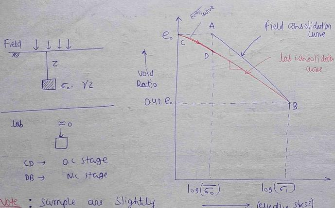
Note: Sample are slightly disturbed when they are taken out from the ground. the disturbance cause a slight decrease in the slope of laboratory consolidation curve
