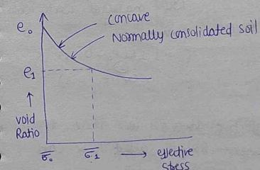
$$\text{slope of eVs } \frac{de}{d\sigma} = \frac{e_0 - e_1}{\sigma_0 - \sigma_1}$$
