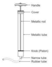
A cycle pump consists of a long metallic hollow tube. There is a small narrow tube connected to one of its ends. A long metallic rod fitted with a rubber knob is passed through the open end of the tube. The rod and the knob are passed in the tube such that the knob is air tight with the tube. This arrangement is called a piston. This rod has a handle attached to the other end of the rod. A rubber tube is connected to the narrow tube.
