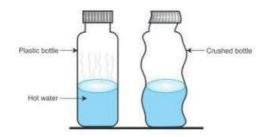
The bottle contracts and is compressed when cold water is poured over it. The closed bottle with hot water contains steam. When cold water is poured over it, the steam inside the bottle cools and condenses. This reduces the air pressure inside the bottle and it cannot balance the high air pressure from outside. So, the high air pressure from outside the bottle crushes it inwards.
