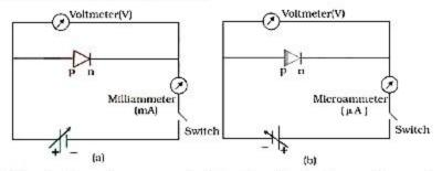
The battery is connected to the diode through a potentiometer (or rheostat) so that the applied voltage to the diode can be changed. For different values of voltages, the value of the current is noted. A graph between V and I is obtained as in Fig. (c).
