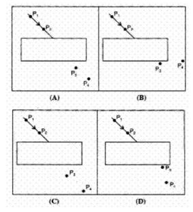
The correct fixing of the pins  $P_1$  and  $P_2$ , for 'defining the incident ray', and of pins  $P_3$  and  $P_4$ , for finding the emergent ray', has been done by student: **(1)**
