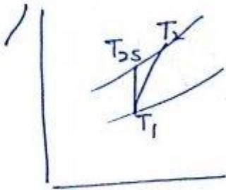
$$\frac{T_{2s} - T_1}{T_2 - T_1} = 0.89$$
