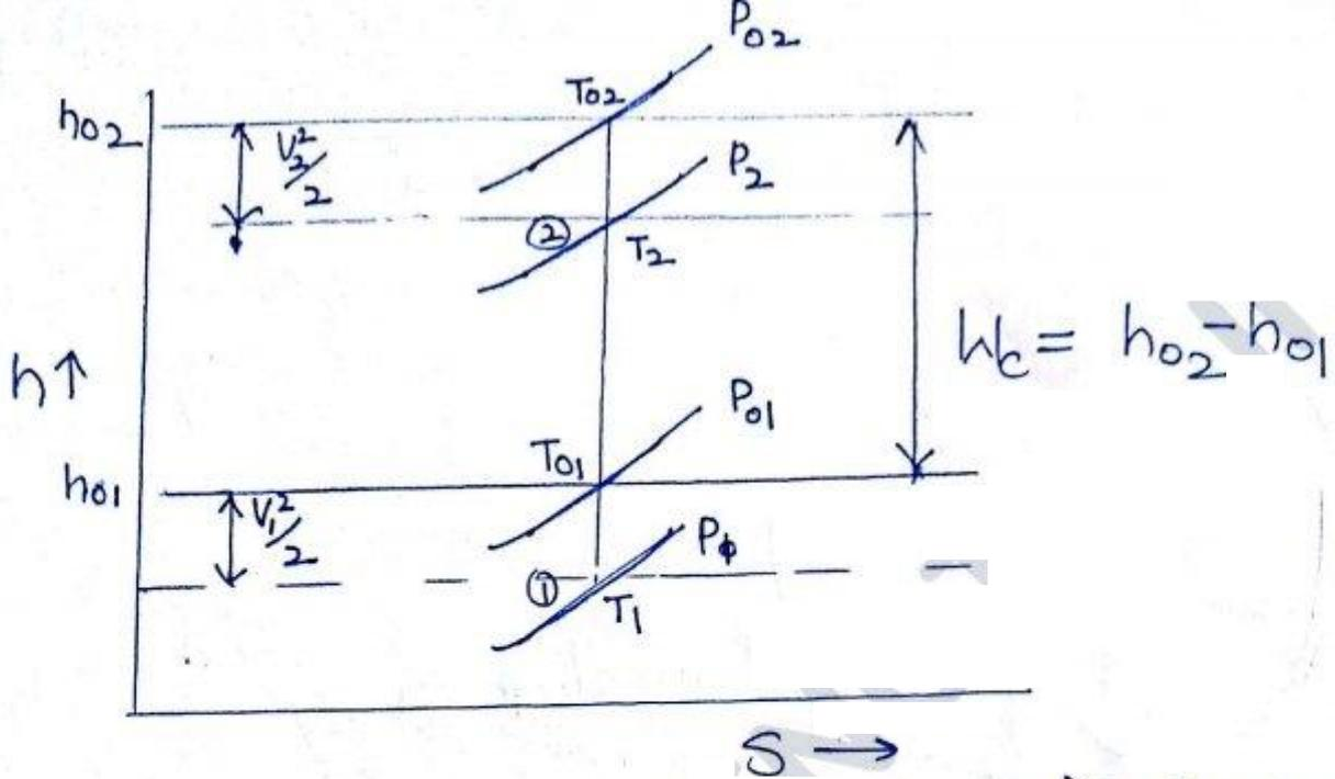
Stagnation state works as a reference point to denote total energy of fluid. Stagnation enthalpy always remains constant for energy transformation process & for energy transfer it may increase for compressor & decrease for turbine.
