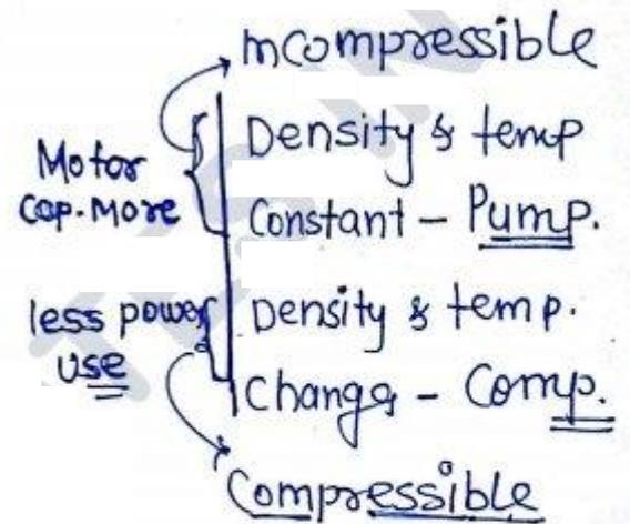
\*The function of a Compressor is to Compress the gases or vapour from a lower pressure to higher pressure and for that work is done from outside.
