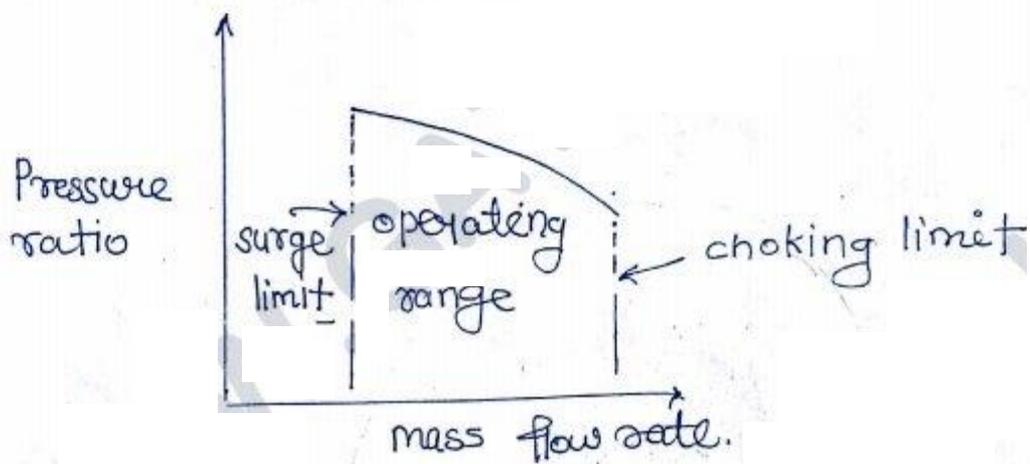
Stalling:- it is aerodynamic flow separation from blade surface due to improper design of blade. It is a local phenomena and the chances of flow separation are more at low mass flow rate, no uniform surface of blade and defect in design.
