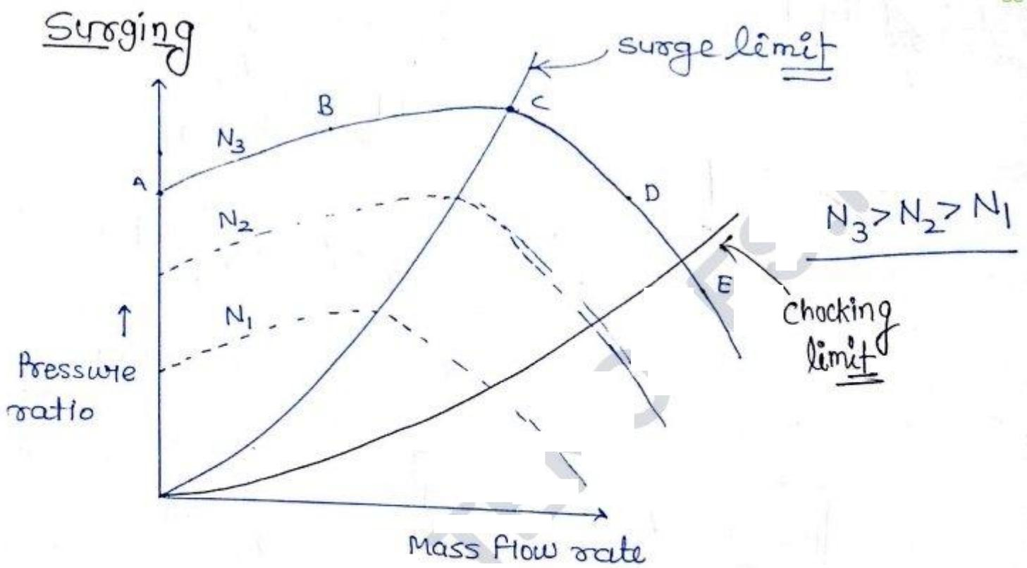
Surging is a complete breakdown of steady flow through the compressor due to periodic flow reversal. This reversal of flow occurs during closing of valve in the operating range having mass flow rate less than corresponding to max pressure ratio. This reversal of flow causes decrease in efficiency, abnormal sound, vibration and the intensity is more. It may lead to mechanical damage.
