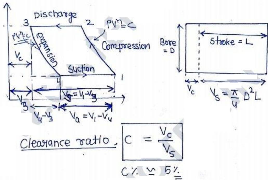
Work input per cycle is given by Area 1-2-3-4-1
