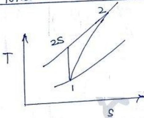
$$\eta_c = \frac{T_{2s} - T_1}{T_2 - T_1}$$
