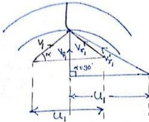
$$V_{r_1}' > V_{r_1} \quad \text{relative Vel.}$$
