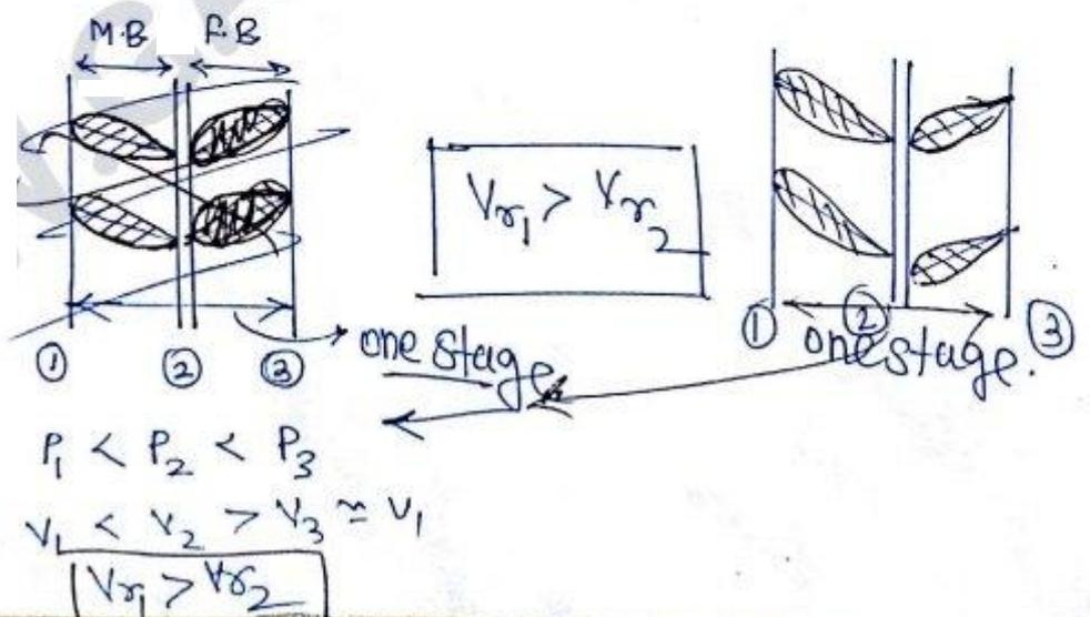
In Axial flow compressor air flow along the axis of rotation and it consist of no of stages. Each stage consist of a set of moving and fixed blade and the cross section between the blade passage is made diverging type both for moving & fixed blade.
