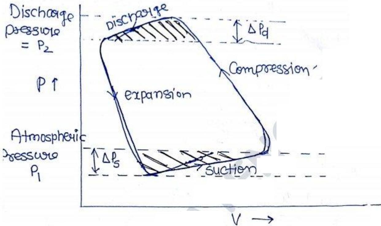
In actual working there is resistance offered by suction & discharge valve due to which actual work input required increases by shaded area.
