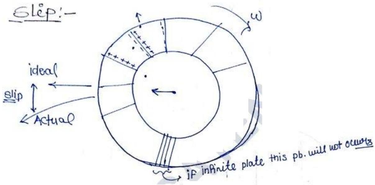
Under ideal condition we assume that the fluid particle exactly follow the blade profile but in actual working where the number of plates are finite air is trapped between the blade passage due to its inertial effect which create pressure diff. across the blade **due to this pressure diff.** fluid deviate from the ideal path and this deviation is called as slip. Due to slip actual blade angle at outlet always decrease which ~~the~~ decreases the whirl component at outlet.
