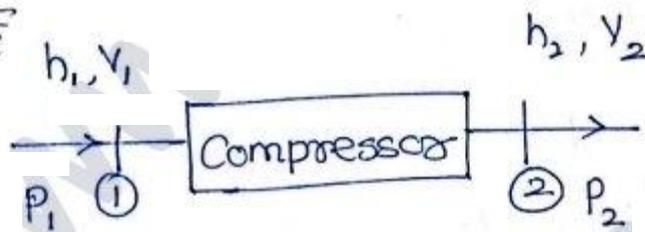
$$\dot{m} \left( h_1 + \frac{v_1^2}{2} \right) = \dot{m} \left( h_2 + \frac{v_2^2}{2} \right) - P_{act.}$$
