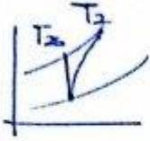
$$\frac{T_{2s}}{T_1} = \left(\frac{P_2}{P_1}\right)^{\frac{\gamma-1}{\gamma}}$$
