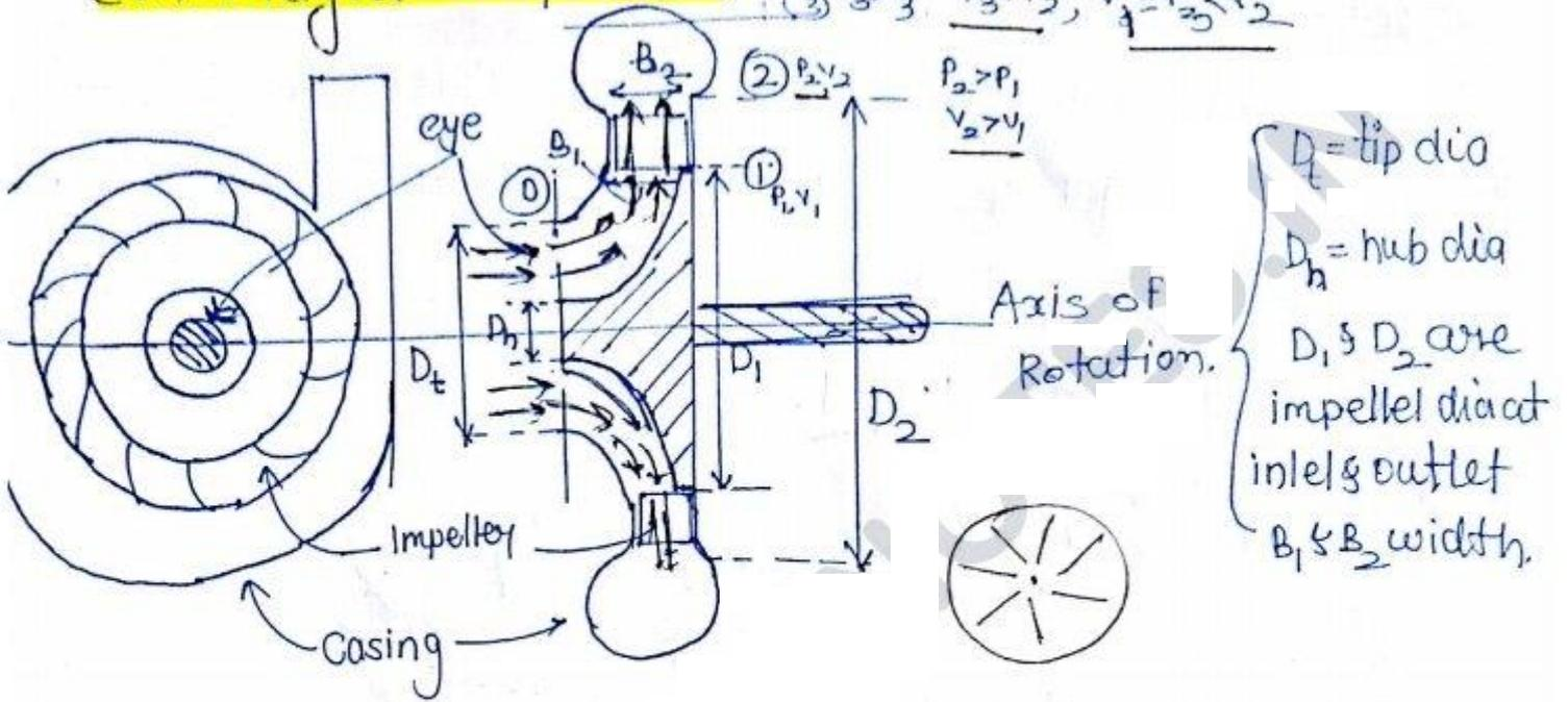
Radial Flow:- while passing through the moving part if flow takes place in a direction  $\perp$  to the axis of rotation it is termed as radial flow machine.
