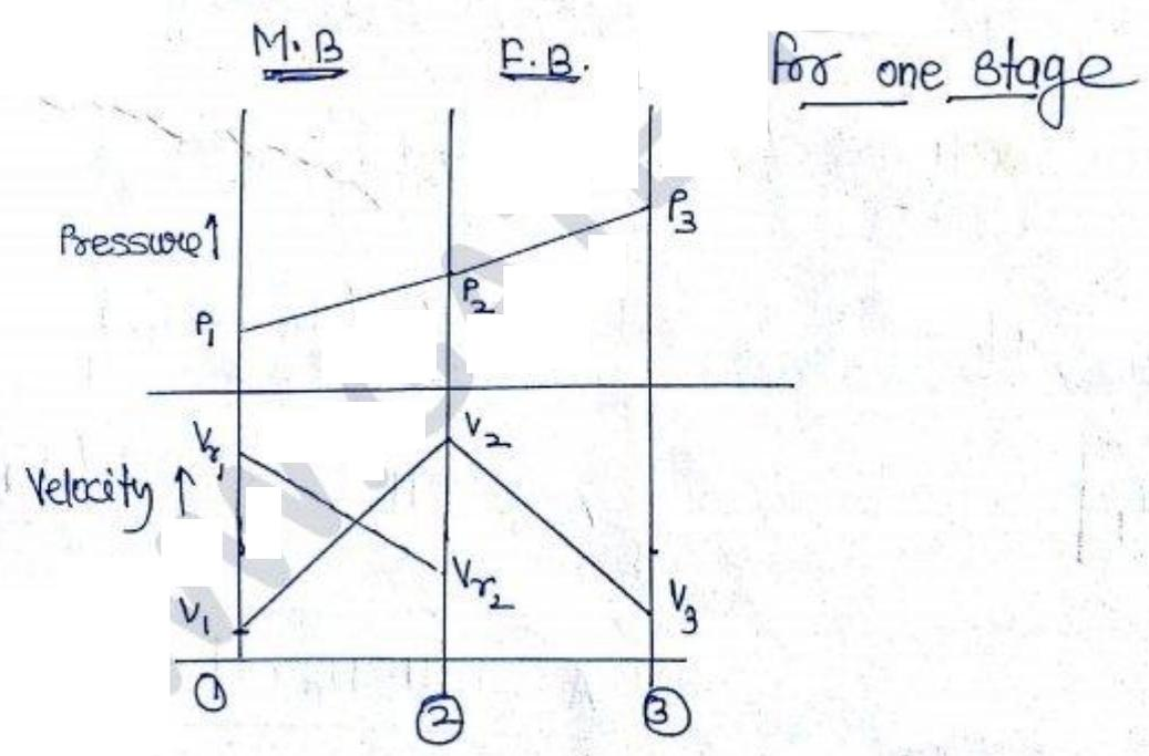
Note: Height of blade is decrease from inlet to outlet as pressure increases to get a constant axial flow velocity in order to neutralise axial thrust on the rotor
