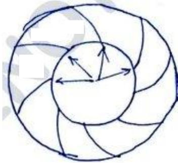
At the inlet to the impeller fluid always enters in the radial direct. i.e.  $\alpha = 90^\circ$  and  $V_{w1} = 0$
