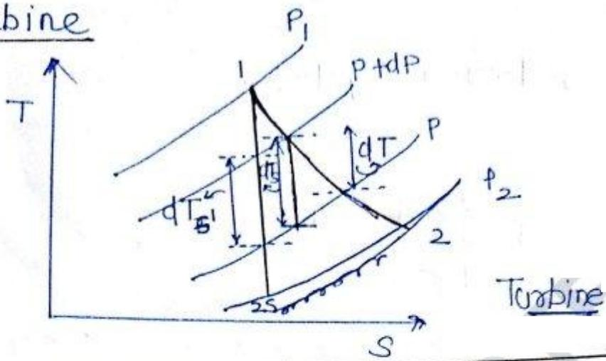
$$\eta_{p,T} = \frac{dT}{dT_s} = \left( \frac{\gamma}{\gamma-1} \right) \left( \frac{\eta-1}{\eta} \right)$$
