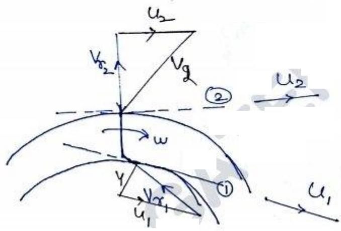
$$u_2 + v_{r2} = V_2$$
