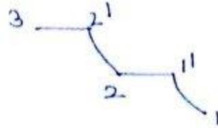
$$(1) \quad W_{\text{cycle}} = \left( \frac{\eta}{\eta-1} \right) m R T_1 \left( \left( \frac{P_2}{P_1} \right)^{\frac{\eta-1}{\eta}} - 1 \right)$$
