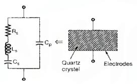
$$z = \left(\frac{1}{j\omega C_s} + j\omega L + R_1\right) \left\| \left(\frac{1}{j\omega C_p}\right) \right\|$$
