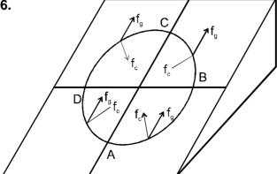
Friction force acting on car will be resultant of the components shown in the diagram.
