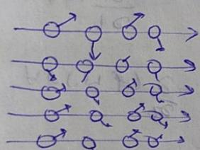
A fluid motion is said to be turbulent when the fluid particle move in an entirely haphazard manner, that result in a rapidly continuous mixing of the fluid. in such a flow eddies of different sizes and shape are present.
