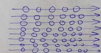
A flow is said to be laminar when the various fluid particles move in layers. when one layer of fluid sliding smoothly over an adjacent layer
