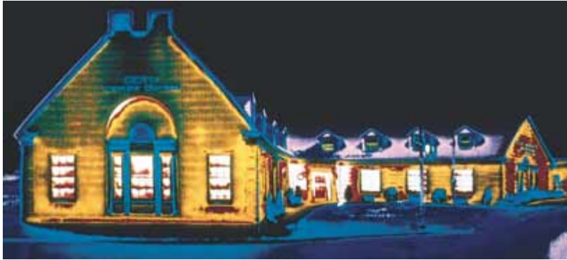
This thermogram of a home, made during cold weather, shows colors ranging from white and orange (areas of greatest energy loss) to blue and purple (areas of least energy loss).
