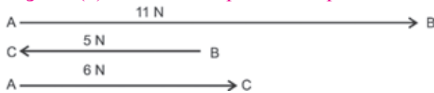
Fig 2.4 (b): Resultant of anti-parallel forces.
