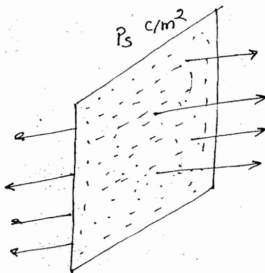
→ The electric field is completely normal to the sheet and the field lines are parallel to themselves
