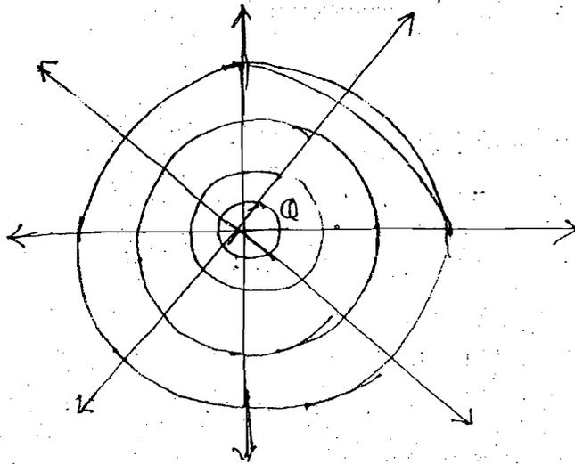
$\rightarrow$  The family of co-centric equipotential surfaces represent the potential distribution and variation of potential in the region and similar to vector intensity line
