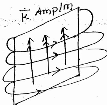
→ The magnetic field is completely normal to the current and the field lines are parallel to themselves and to the sheet
