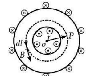
So, the magnetic field is only confined inside the body of a toroid in the form of concentric magnetic lines of force.
