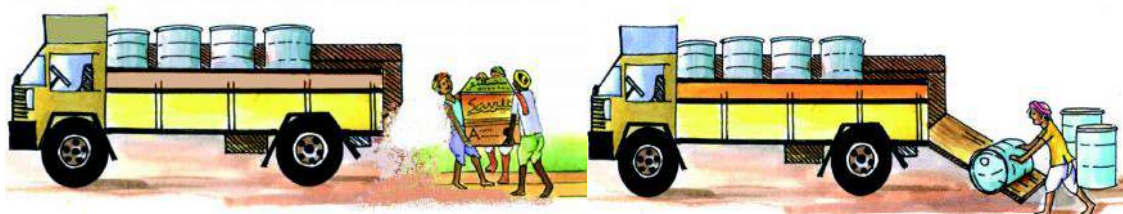
b. Raising using an inclined plane
